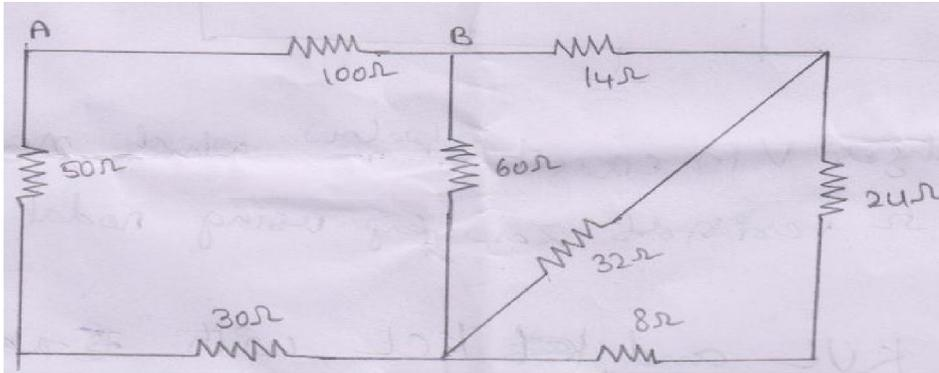
12. Determine the current delivered by the source in the circuit shown?
