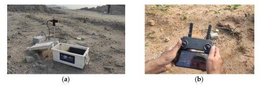
Figure 14. (a,b) NOMIS seismograph and satellite-based DJI remote controller.
