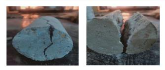
Fig. 4 Cylindrical tested specimens for split tensile strength
