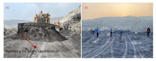
Figure 9. (a,b) Bench leveling and preparation for drilling.
