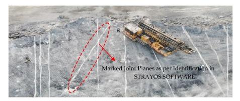
Figure 10. Bench-joint planes marking.
