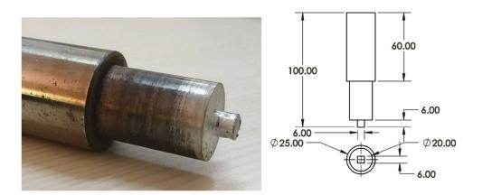
Fig. 1 Photograph and the dimension of FSP tool (all dimensions are in mm)
