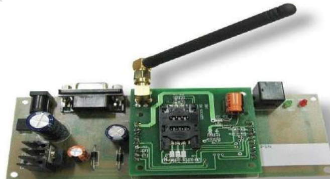
Fig.1 GSM board with slot for sim card.
