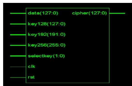
Figure 3. Schematic Diagram AES-128/192/256 Architecture
