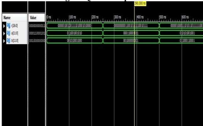
Fig.5. Simulation result of Signed QSD multiplier.
