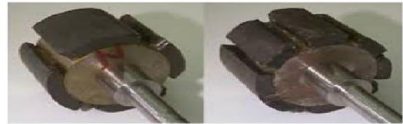
Fig.2 BLDC motor Rotor construction
