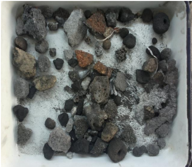
Fig: 2 Deleterious Materials in WFS
