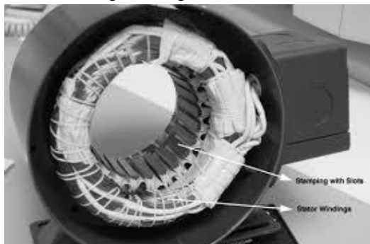
Fig.1 BLDC motor stator construction
