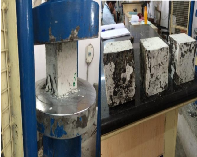
Fig: 4 Cube specimens under test
