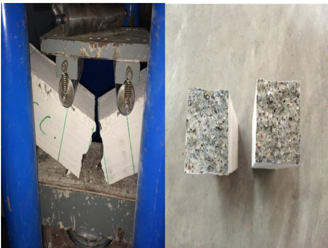
Fig: 5 Flexural beam specimens under test
