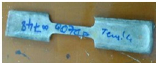
Fig 5. Laminate as per dimensions according to ASTM standards.
