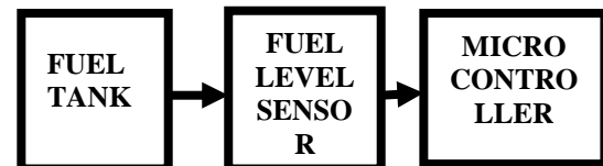
Fig. 1 Block diagram of level sensing unit
