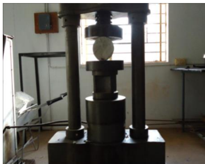
Figure 4 Illustration of compressive strength testing machine with cylindrical shape binary concrete.
