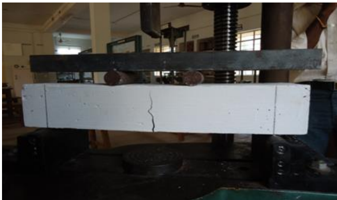
Figure 4 Illustration of fracture of failure specimen.
