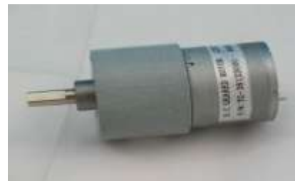
Fig 3.4 Motor to drive the robot
